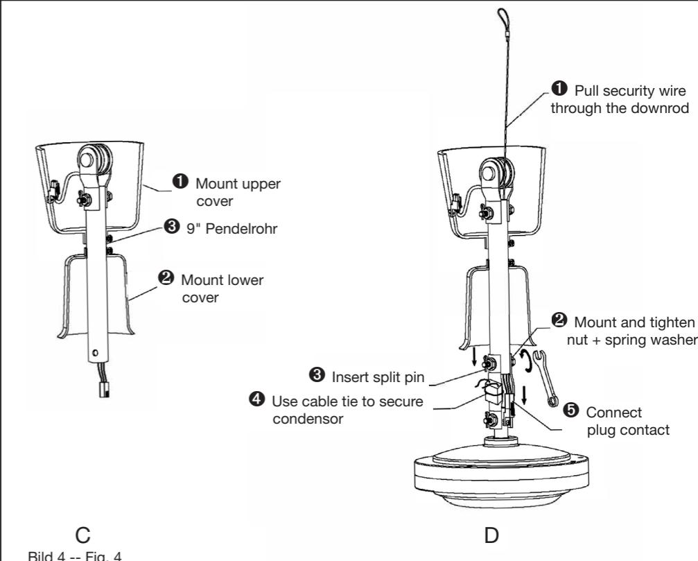
Note: The drop height must be taken into account for the security wire.
