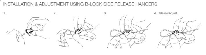
Ensure a minimum 75 mm of tail wire exits the hanger.
