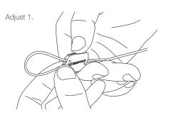
Ensure a minimum 75 mm of tail wire exit the hanger.
