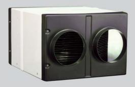
A ducted heat recovery unit for residential or commercial applications. The HR200V is self-contained and includes two mixed flow speed controllable fans. Using a high performance, polymeric heat exchange cube together with two power fans, the HR200V can boast a temperature efficiency of up to 70%. Low speed for trickle ventilation mode.
