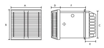
Wall fixing hole 250mm x 250mm sq.
